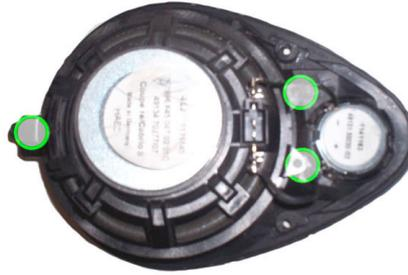
If your car is fitted with a tweeter as well as the main speaker, you will need to cut the wires to it, or remove the tweeter with the main speaker. If you remove the tweeter we recommend you make the grill aperture air-tight using adhesive tape.
