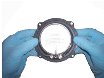
Place the speaker into the grill, lining up the notch on the ring with the raised flat upright of the grill as seen in this picture.
