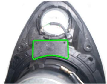
Attach the wiring adapter as shown in this image. the adapter will only connect to your speaker in one orientation.
